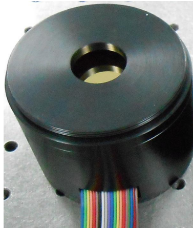
Figure 2. Photograph of the assembled unimorph DM.
