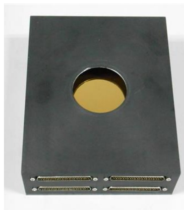
Fig. 4 The packaged double drive modes unimorph DM.
